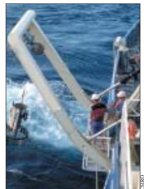
Marine scientists water sampling Australian oceans to determine salinity, temperature, dissolved oxygen.
